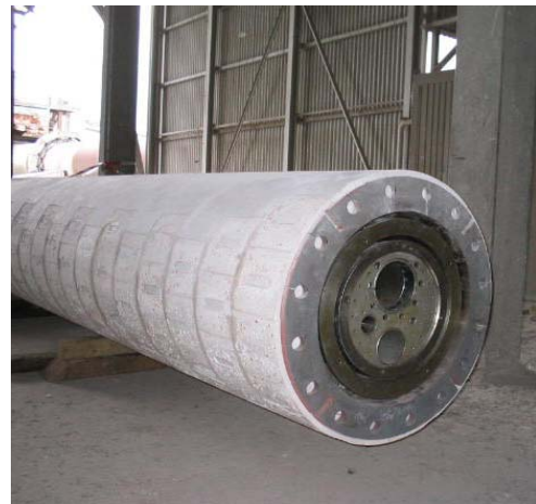
MAS multifuel kiln burner covered with ceramic bricks on the jacket tube to enlarge the lifetime of the heat insulation.
