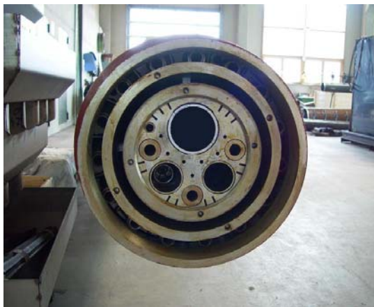
MAS/5/KO.EG.SO.X Burner for LAFARGE Beocin in operation with 100% petcoke or 100% anthracite
