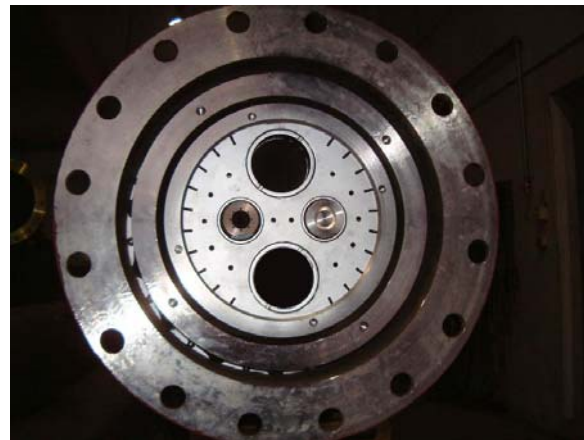
MAS/6/KO.SO.X Burner for HOLCIM Koromacno in low NO x technology for 5 different fuels
