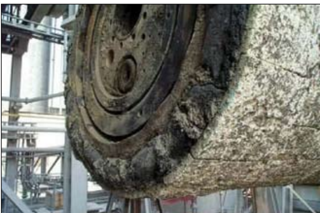
Figure 3 (above) and 4 (below). No significant wear of burner refractory after six months operation.
