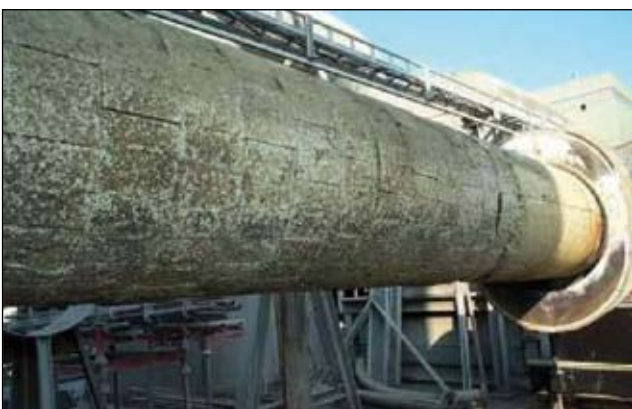
Figure 3 (above) and 4 (below). No significant wear of burner refractory after six months operation.
