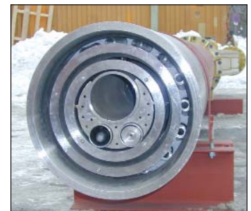
Figure 6. M.A.S. kiln burner for secondary waste fuels.
