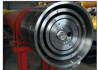
Figure 2. Combined M.A.S. kiln burner for coal, heavy oil, gas.
