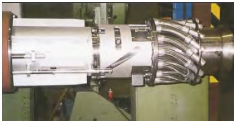
Figure 3. Burner front without frontier jacket tube, showing the swirl setting device.
