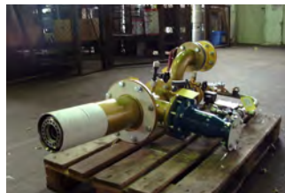
Combined Calciner Burner
