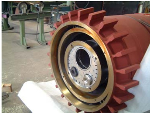
M.A.S burner with cast iron ribs on the divisible burner jacket tube to enlarge the refractory lifetime
