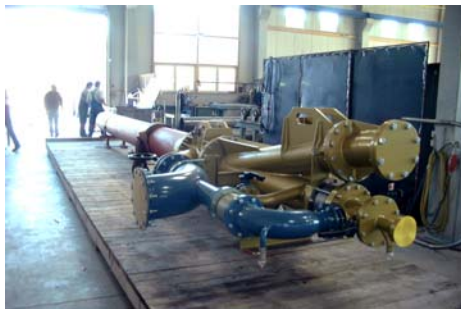
Left: M.A.S kiln burner at the shop-inspection for the contract with Zaman Cement
