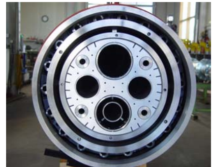
Combined M.A.S. kiln burner for Prachovice Cement, for three traditional fuels and three alternative fuels.
